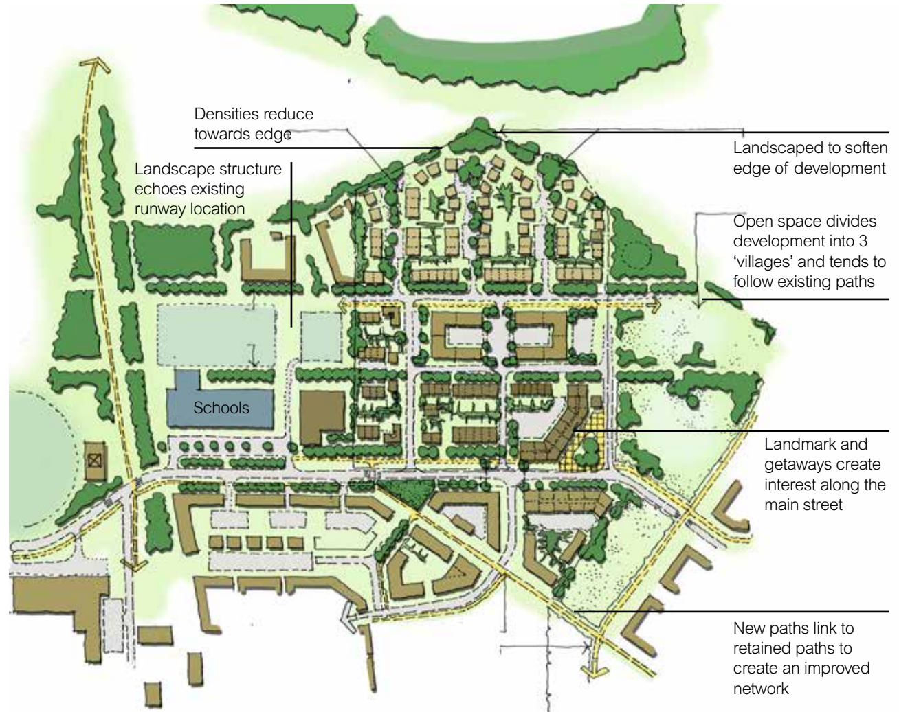
Fig 64: Illustrative drawing showing how residential density in Wisley reduces towards the edge of the site.
