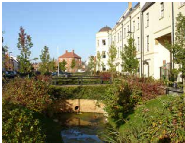
Formal swales incorporated within an urban context, drawing green infrastructure into the streetscape.
